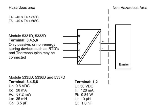
**CLASS 2258 04 - PROCESS CONTROL EQUIPMENT** - Intrinsically Safe Entity - For Hazardous Locations
